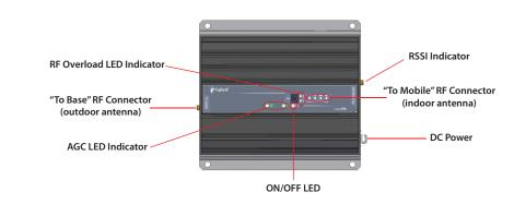
• RSSI Indicator: Shows the level of the received signal from the cellular site, and helps to fix the outdoor antenna in the proper position to provide the best possible indoor coverage.
