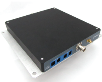
Transmitter Bypass (TXBP)
