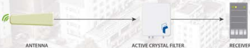
Active Crystal Filter application at a single Receiver, with direct connection to the Rx antenna
